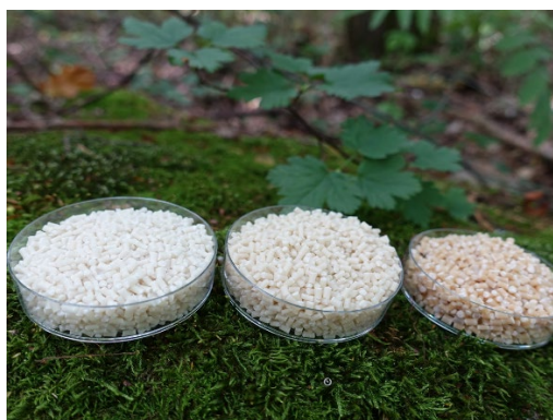
Figure 1. 3D-printable cellulose-based composite material
