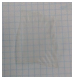
Figure 1. Kraft pulp cellulose films crosslinked with epoxides.
